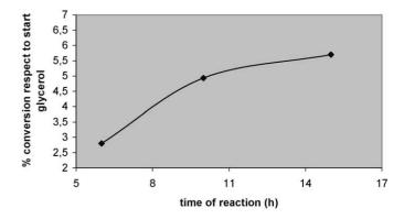
Fig. 1. Trend of conversion of glycerol into glycerol carbonate with  $n-Bu_2Sn(OMe)_2$  as catalyst. [PCO<sub>2</sub> = 5 MPa, 450 K].
