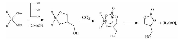
Scheme 2. Reaction mechanism of formation of glycerol carbonate from glycerol and CO<sub>2</sub> under n-Bu<sub>2</sub>Sn(OMe)<sub>2</sub> catalysis.
